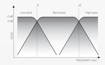
What kind of frequency crossover is used depends on the driver system. Therefore, the filter rate, the frequency of the loudspeaker as well as its phase has to be considered at the same time. Furthermore, the resistance of the loudspeaker, depending on the frequency, has a detrimental effect on the operation of the frequency crossover.
