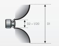
At a given SPL output a horn loaded driver can be designed significantly smaller than a driver without a horn. This results in a reduction of the moving mass of up to 1/20!
