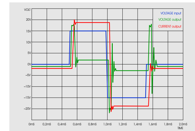
Fig. 2: iTRON current amplifier simulation
