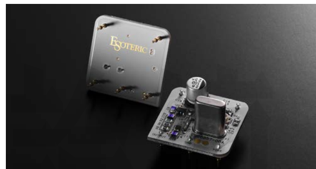
● K-01XD SE特別訂製的Master Sound Discrete Clock
